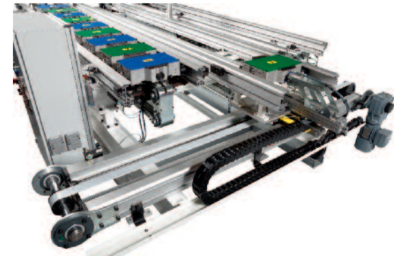
Detail of distributing station for 3 component types
