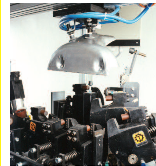
System for joining the cover sheet of an exhaust manifold
